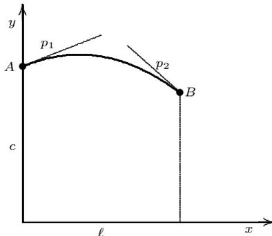
The problem is to determine the maximum height of the bridge as a function of the parameters mentioned above. In order to set up the solution we must use some notions of analytic geometry which we will assume are known.
